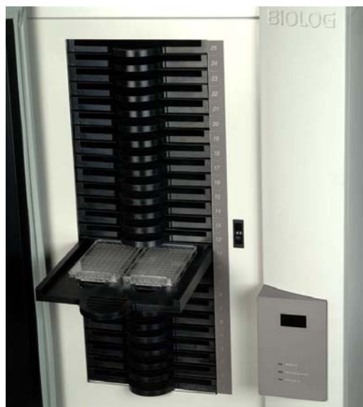
OmniLog with PM Panels in the OmniLog Shelves Capacity 50 Standard MicroPlates
